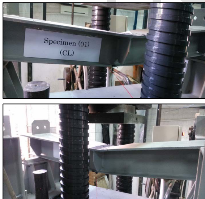
Fig. 8. Failure mode of control beam (CL)
