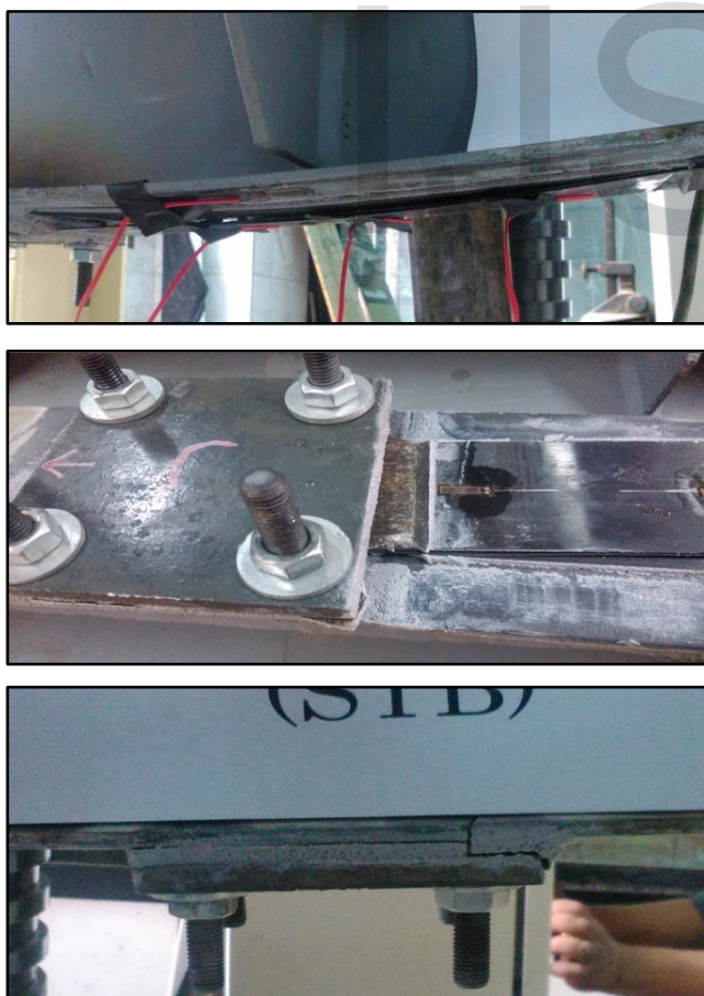
Fig. 11.Failure mode of STB beam
