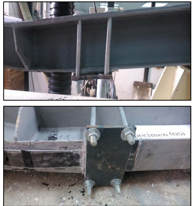
Fig. 12.Failure mode of STC beam
